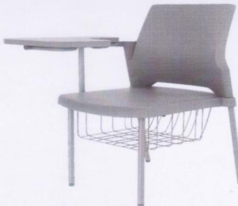
The Seat and Back should be made up of injection moulded indoor grade PolyPropylene compound SEAT SIZE : 52.5 cm. (W) x 53.2 cm. (D) BACK SIZE : 51.6 cm. (W) x 40.5 cm. (H) The powder coated ( DFT 50±10 microns ) welded tubular frame should be made from 0.222 ± 0.03 cm x 0.16 ± 0.0128 cm and 3.5 ± 0.03 cm x 1.5 ± 0.03 cm x 0.16 ± 0.0128 cm MSERW tube.
